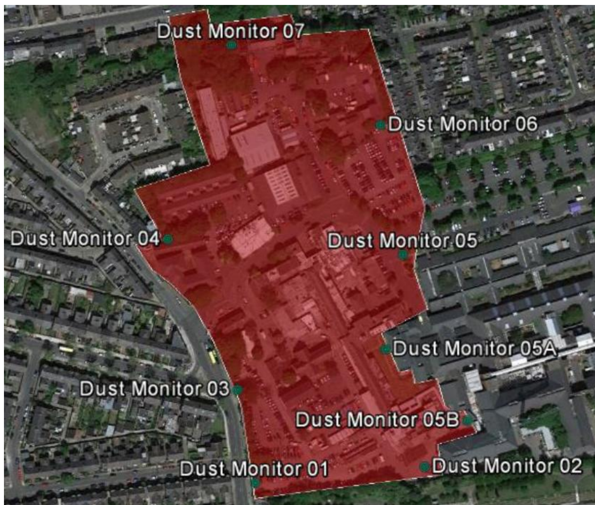
Figure 2. Previous location of Dust monitors on site (April 2017 to August 2017).
