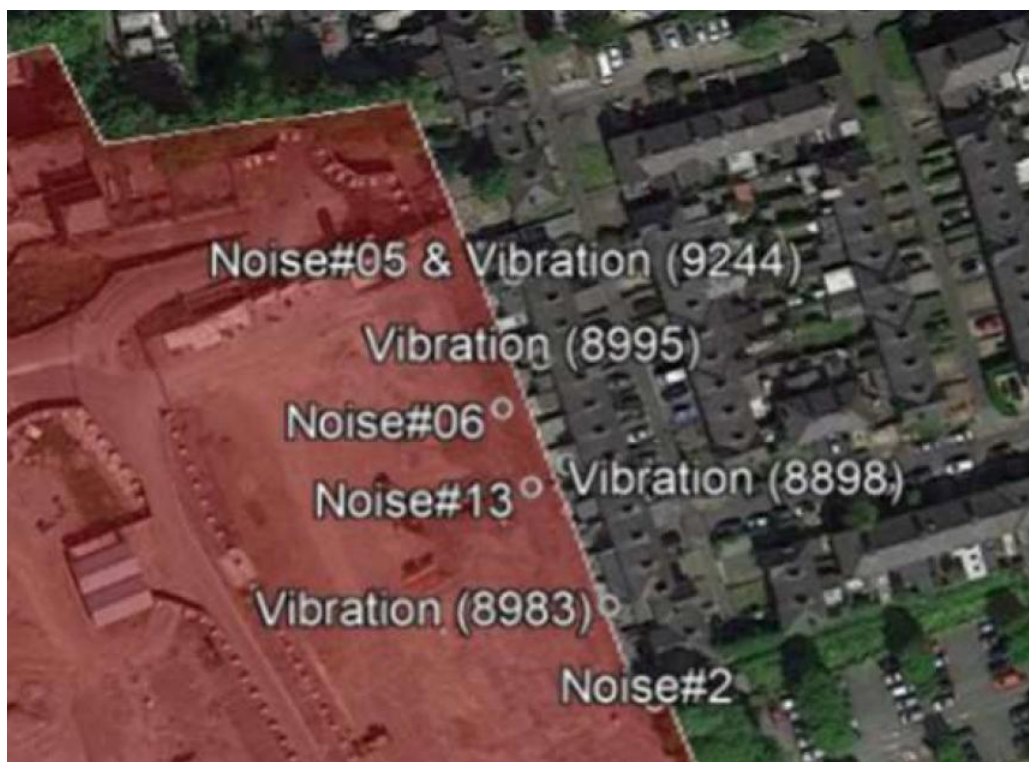
Location of Vibration Monitors around O'Reilly Avenue
