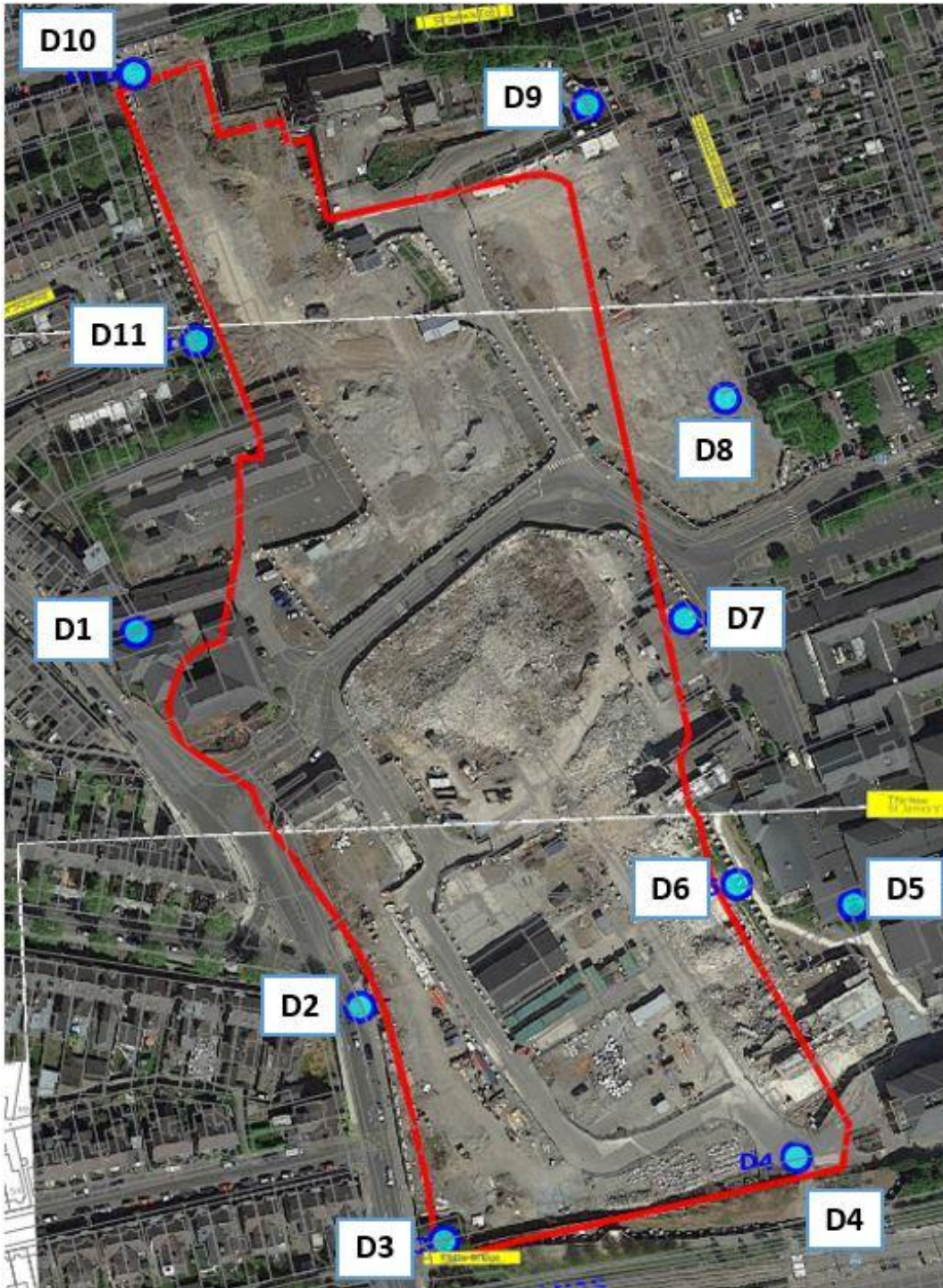
Figure 1. Location of Dust monitors on site (December 2017).
