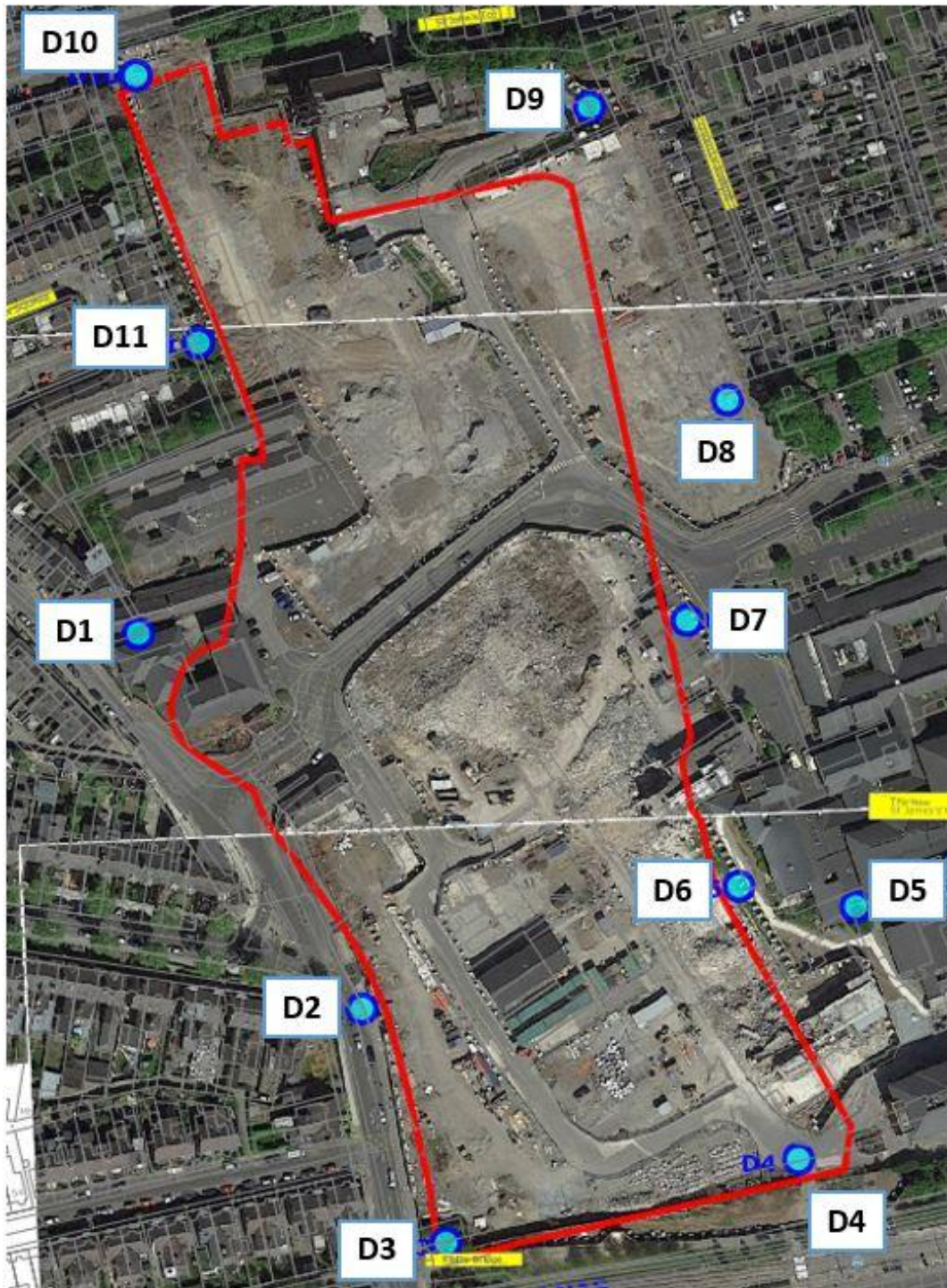
Figure 2. Location of Dust monitors on site (September 2017 – April 2018).
