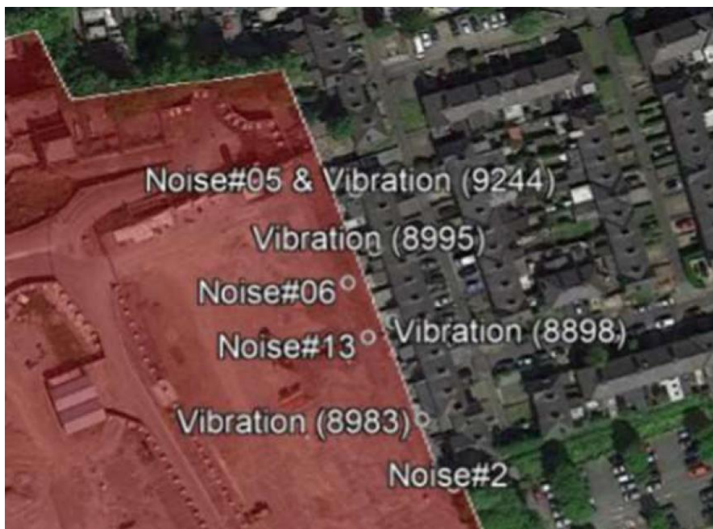
Location of Vibration Monitors around O'Reilly Avenue
