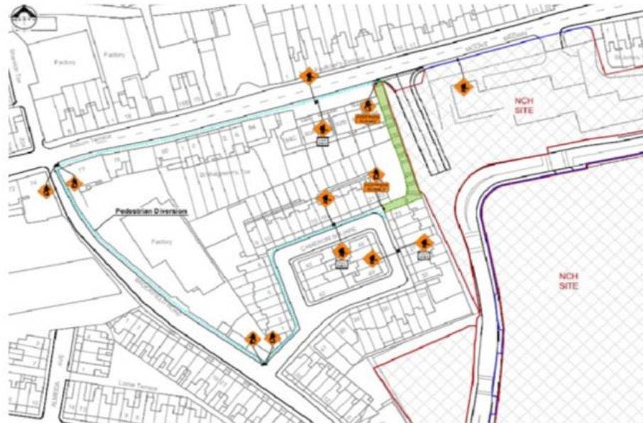
National Childrens Hospital - Public Realm Update Mt Brown Steps - Traffic Management Plan
